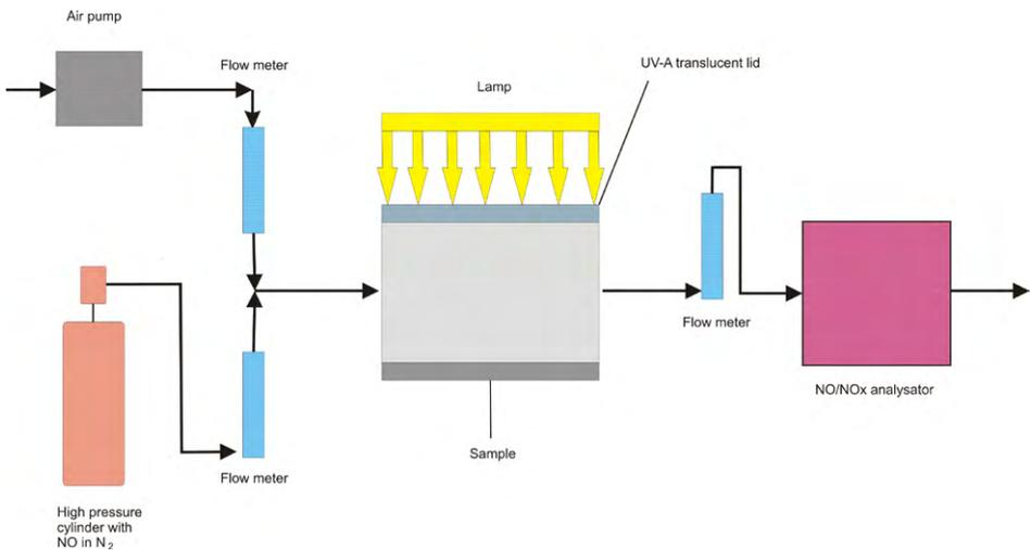
Fig. 4. Scheme of testing equipment for NO<sub>x</sub> as in standard 11247:2007
