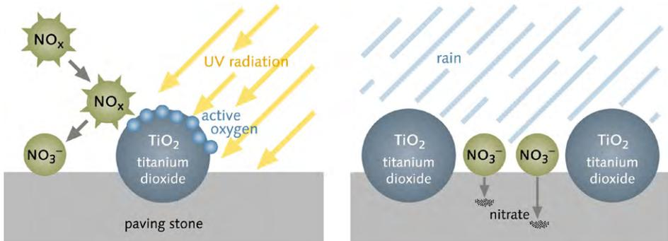
Fig. 7. Reaction process – How TioCem reduces NO<sub>x</sub>
