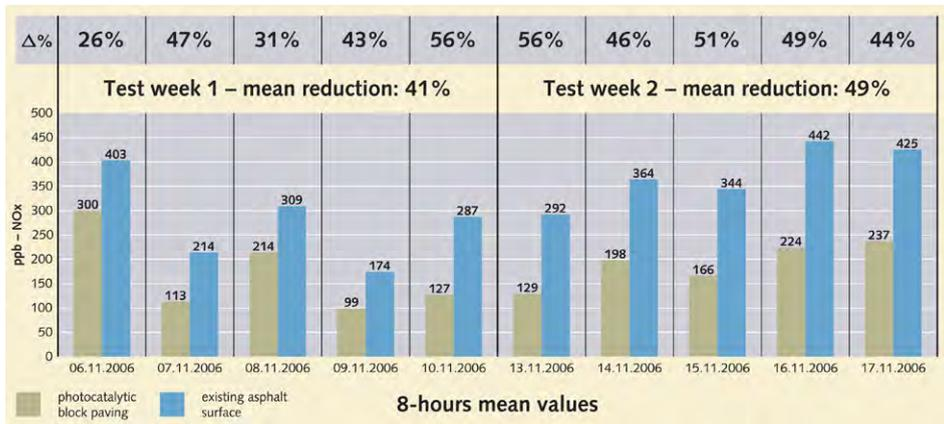
Fig. 6. Via Borgo Palazzo NO<sub>x</sub> reduction; mean values measured in the period of 8 hours (9:00 – 17:00)<sup>7</sup>
